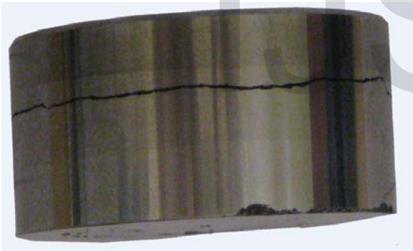
Figure 2.1 Cracking of metal-ceramic FGM due to thermal residual stresses
